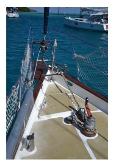
•Primary Anchor: 35 kg CQR anchor, 50 m, 10 mm anchor chain plus 20 m anchor rope for extension, extra chain to attach secondary anchor to primary chain
